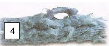
> Image 4 Strand reduced by 25% abrasion
