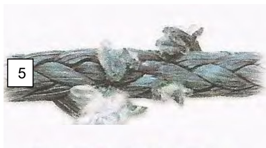
> Image 5 Rope displays two adjacent cut strands.
